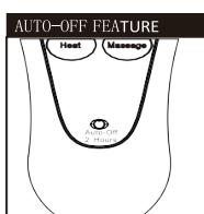
The auto-off feature is included in the control on the heating pad. The auto-off allows to conserve energy by turning off after 2 continuous hours of use. The massage feature will automatically shut off after 15 minutes of use. **IMPORTANT:** the auto-off timer will reset after a power outage.
