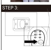
Turn on the switch of the controller's backside and then select the desired heat or massage function on the front of the controller. **IMPORTANT:** if the heat indicators do not light up or stay on, unplug from the electrical outlet.
