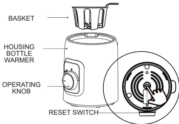
The **reset switch** is used to shut off the power to prevent overheating when the water dries up. Wait 10 minutes or pour cold water into the bottle warmer to cool it down and then press the reset switch (until you hear a clicking sound) to turn the power back on. Then select the function as needed for warming up the baby food.
