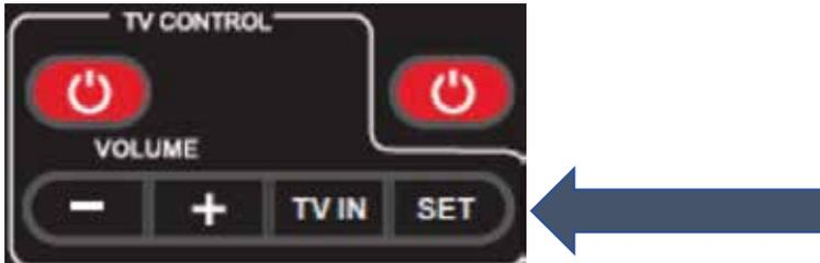
2. Press the "POWER" key on the TV CONTROL area in 10 seconds the red light flash.
