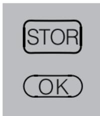
briefly press the **STOR** button and repeatedly press the **OK** button until 'SERVICE ACCESS' appears in the display
