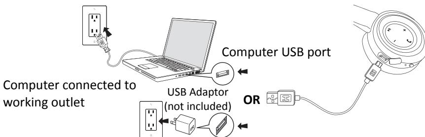
1. Connect the micro USB plug on the charging cable to the micro USB port on the headphone.
