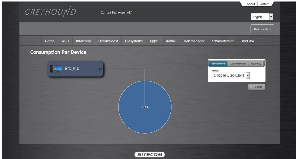
Here you can view the bandwidth consumption per device. You can click on the device to highlight it. You can select the time frame from the drop-down menu.
