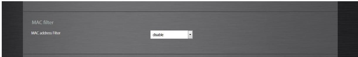
This wireless router supports MAC Address Control, which prevents unauthorized clients from accessing your wireless network.
