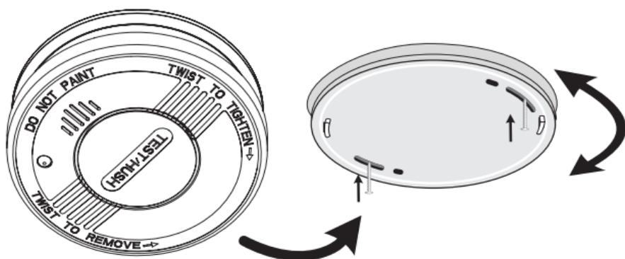
**IMPORTANT:** For optimal operation, we recommend mounting the smoke detector on the ceiling. See also the installation instructions. If ceiling mounting is not possible, we recommend that you place the smoke detector in the middle of a wall. The installation location must be in the natural airflow of the room and free of side walls or slope.
