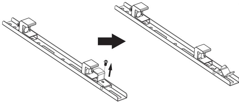
Remove the screws on the adapter brackets and keep the screws for later use.
