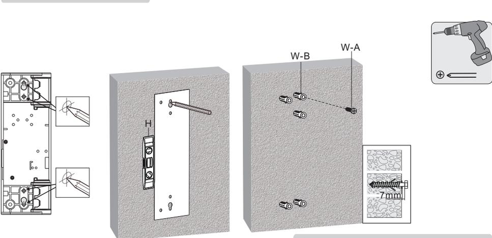
Tighten the screw leaving a 7mm space from the wall.
