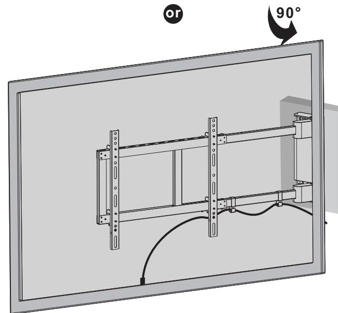
Connect the cables to your TV and route through the cable clips.
