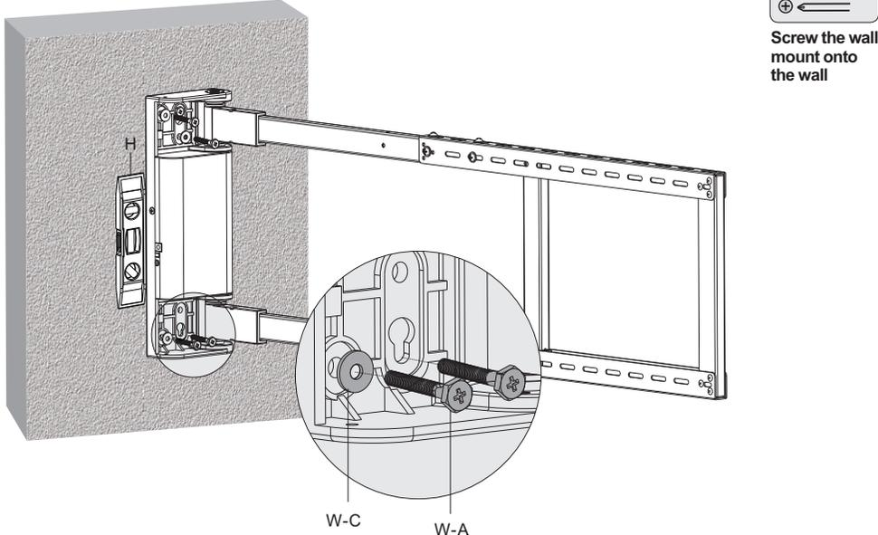
Screw the wall mount onto the wall
